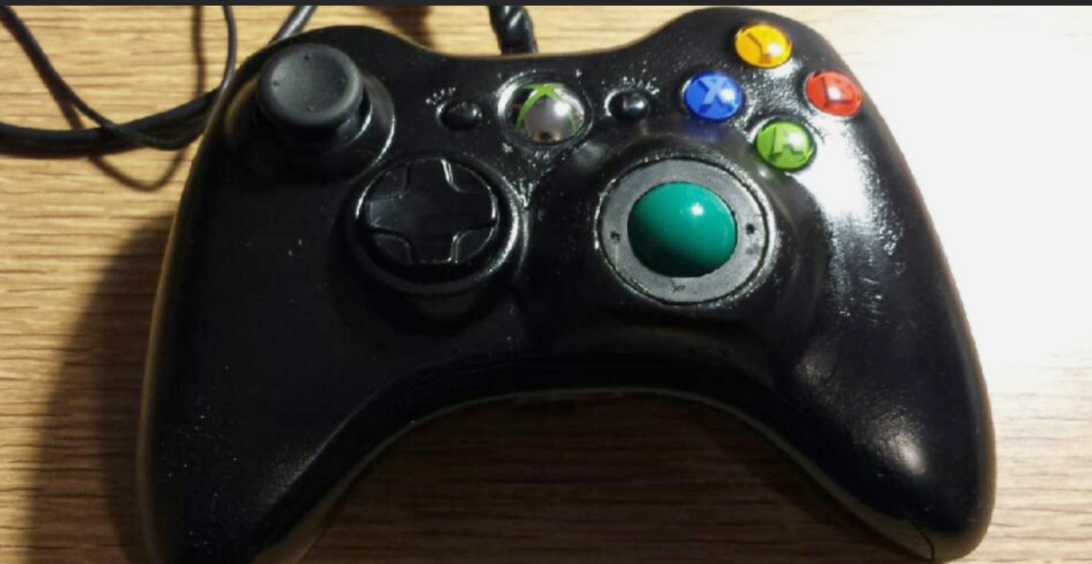
Pictured above: Modified Xbox Controller (Trackball)
